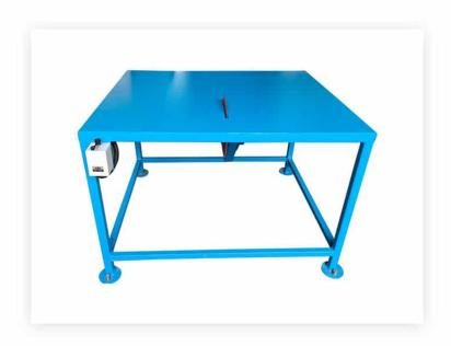
It is used to cut the Plastic lengthy wastages or Plastic rejected components in no. of pieces.
